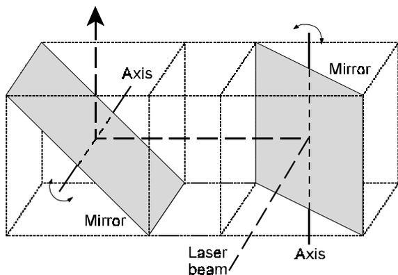
**Fig. 3.1.2** The oscillating mirrors
