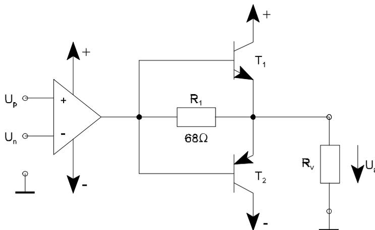
Fig. 3.4.2 Operation amplifier with complementary emitters
