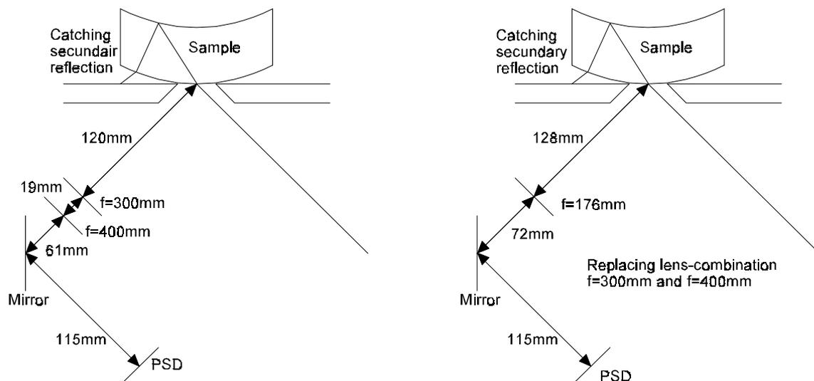
**Fig. 3.1.6** Replacing the lens-combination
