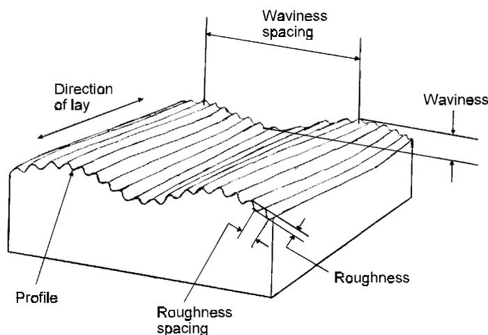
**Fig. 2.2.1** Surface characteristics
